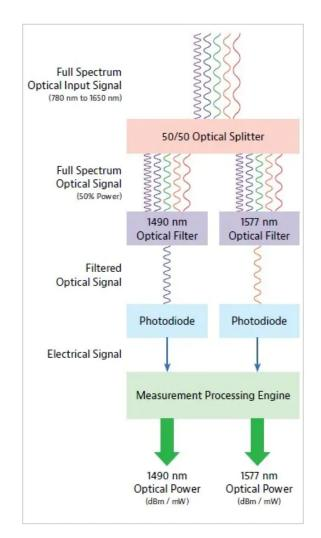
Figure 2. Selective optical power meter schematic.
