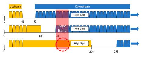
Figure 3. Signal leakage with high split.
