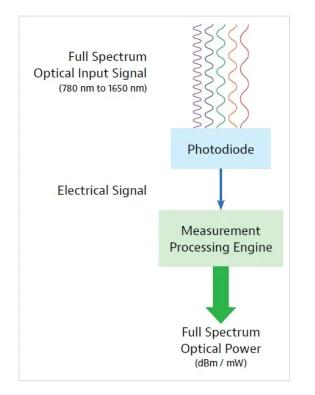
Figure 1. Broadband optical power meter schematic.
